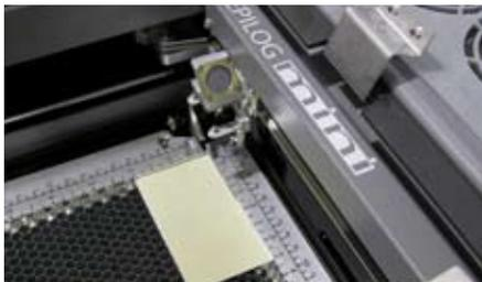
**Step 2)** Place your metal part on the engraving table and “print” your job to the laser. The laser is connected to your PC computer through an Ethernet or USB connection just like a paper printer, but instead of putting ink on paper, the laser engraves onto the surface of the material being processed. Since the laser system acts like a printer, you can use a wide variety of
